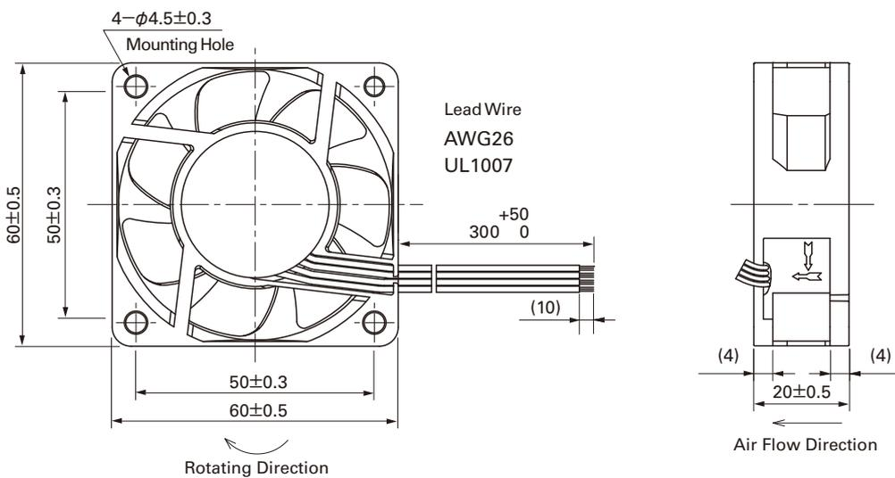
Reference dimension of mounting holes and vent opening (Unit : mm)
